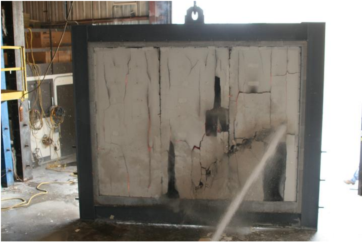
Figure B- 9. Exposed Face at Start of the Hose Stream Test.
