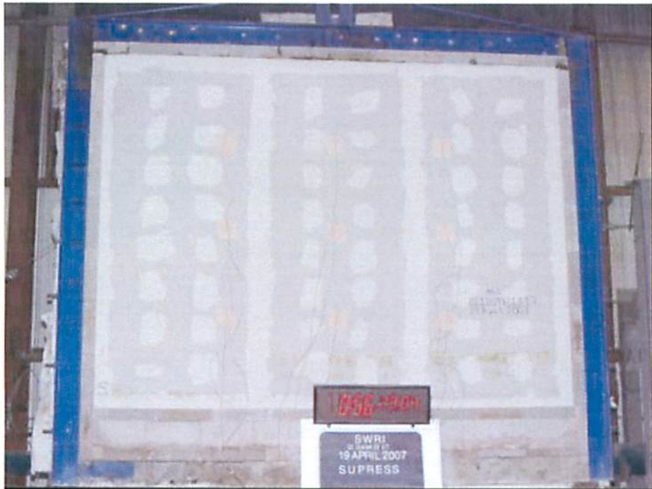
Figure A-2. Unexposed Side of Assembly During the Fire Test.
