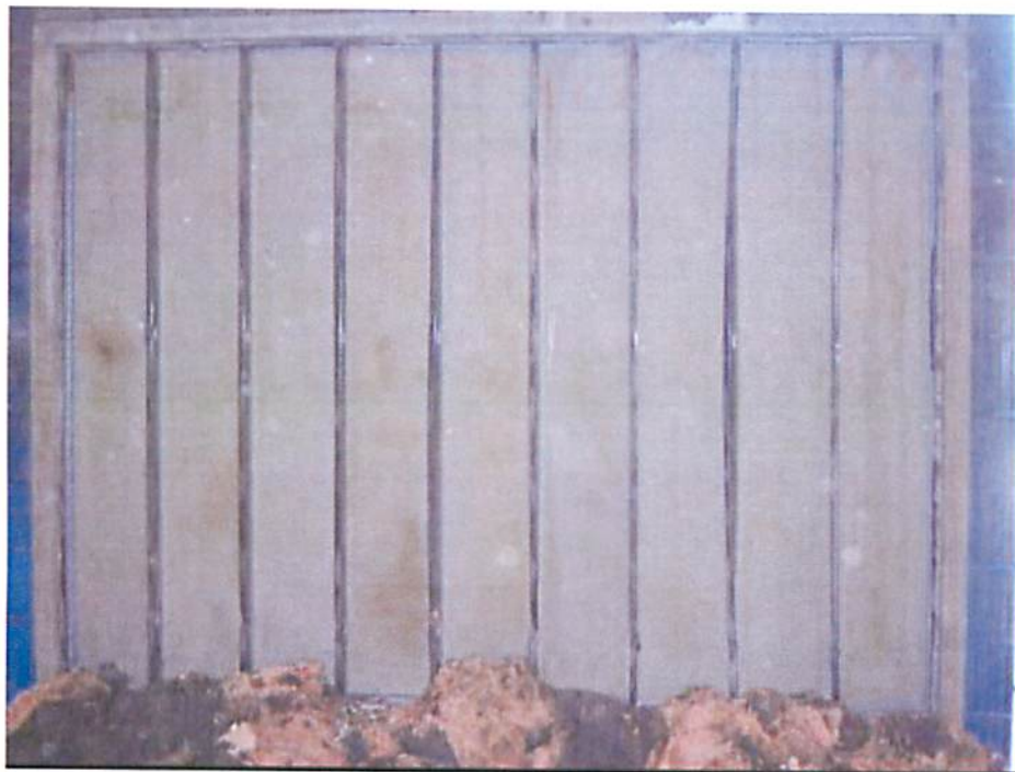
Figure A-8. Exposed Side of Hose Stream Retest Immediately After Hose Stream Test.
