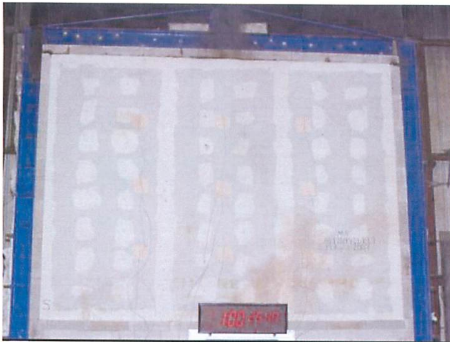
Figure A-4. Unexposed Side of Assembly Immediately After the Fire Test.
