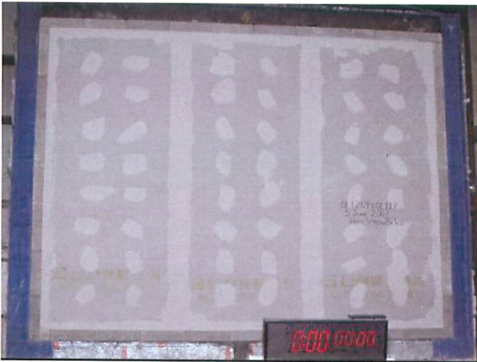
Figure A-6. Unexposed Side of Hose Stream Retest Prior to the Fire Test.
