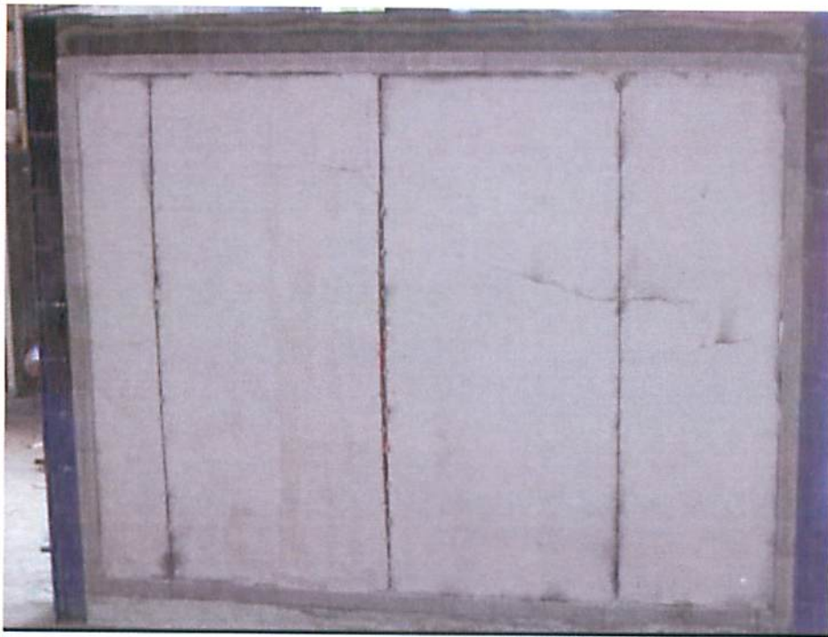
Figure A-7. Exposed Side of Hose Stream Retest Immediately After the Fire Test.
