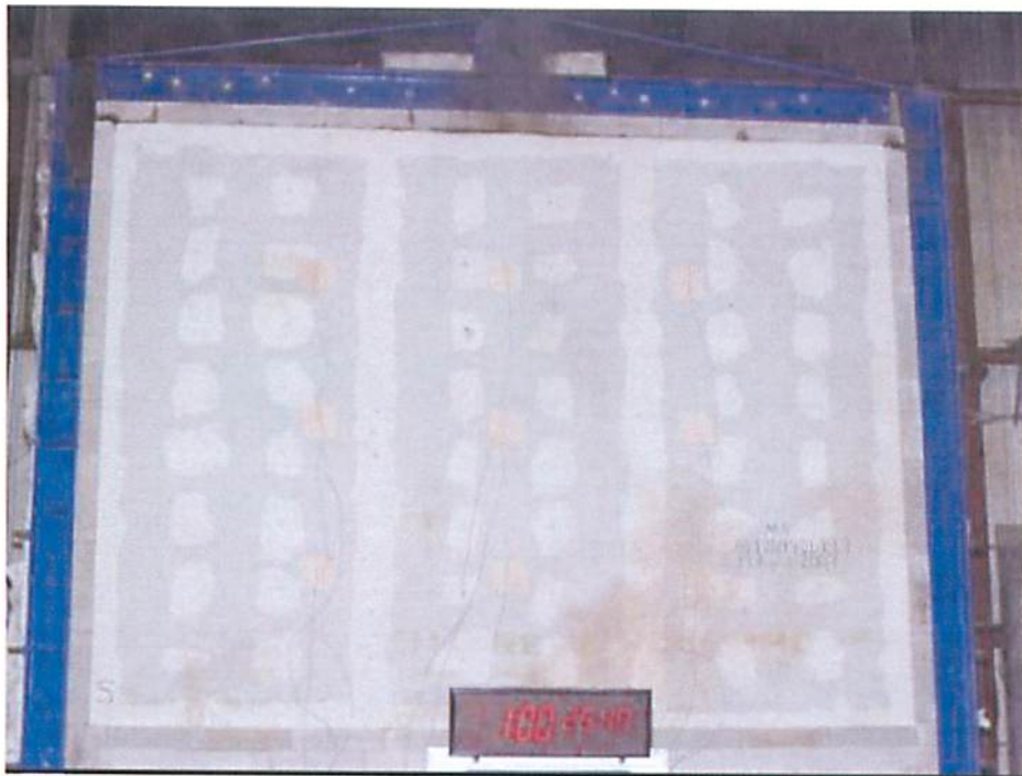
Figure A-4. Unexposed Side of Assembly Immediately After the Fire Test.
