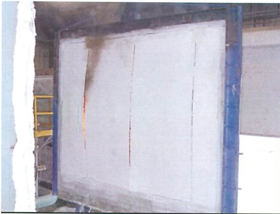
Figure A-3. Exposed Side of Assembly Immediately After the Fire Test.
